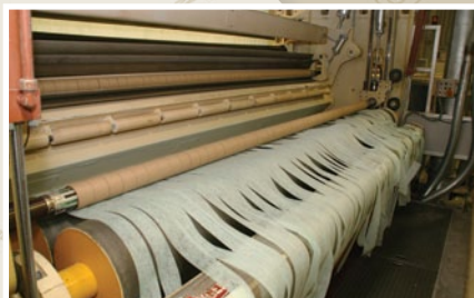
Locked-core shaft in two-drum winder
